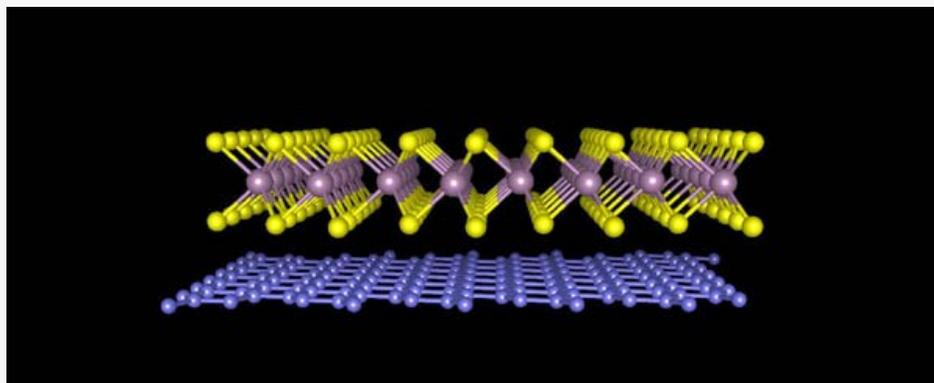
Above, a computer image of research efforts at the University of Kansas to connect atom sheets of tungsten disulfide and graphene thereby forming an entirely new material that has shown much promise.
