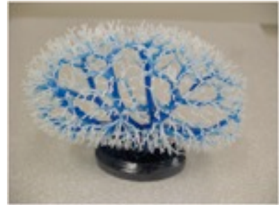
Kidney vascular tree made of plastic using rapid-prototyping techniques ( Bill Beaver, York Technical College )
